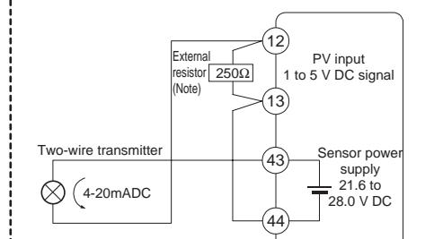
Note : Connecting a 250Ω resistor to the terminals is optional.
